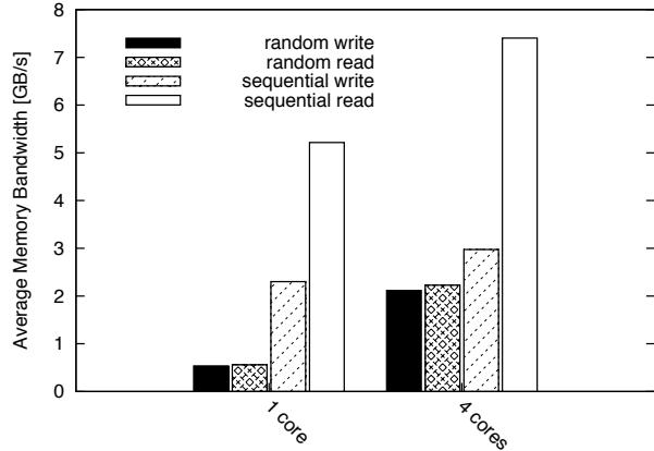
**Figure 1:** Measured memory bandwidth on a quad-core CPU for different access patterns.
